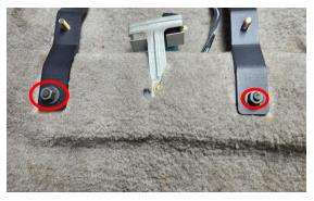
9. Using the factory hardware from step 4, secure the rear of the new Stifflers seat rail extenders. Torque to 25-34 ft-lbs.
