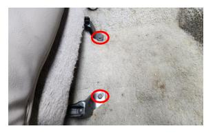
5. First, be sure to unplug the factory power lumbar connector under the seat. Now you can remove seat from the vehicle.
